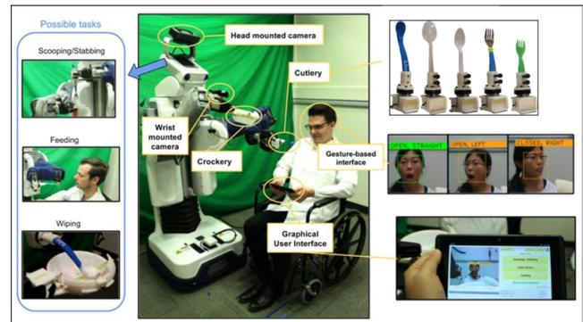
Fig. 1: The outline of a robot-assisted feeding system.
